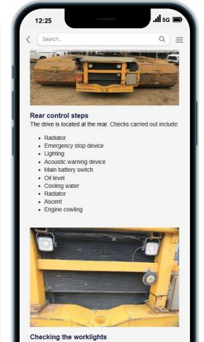
Check the glass of the headlights, as well as the anchoring and position of the headlights.
